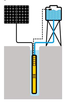
control pump start and stop, connecting a float switch, for example. All the protections against overload, surges and dry running are integrated into the on-board inverter.
