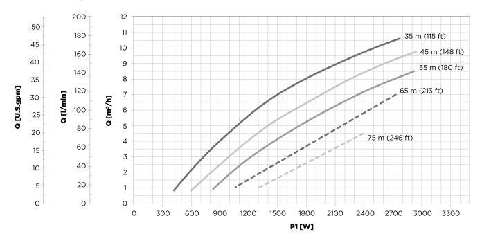
${\sf CM}\ {\sf MultiPower}\ in stallation\ is\ recommended\ for\ points\ of\ operation\ on\ the\ dashed\ lines.$
