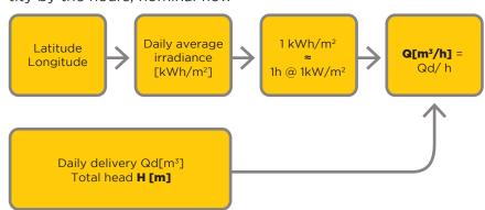
For a full sizing of your solar pumping system, it is recommended using Nastec Solar Calculator (NSC) at:
